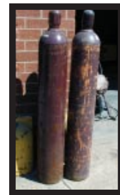
LP Tanks for Forklifts
